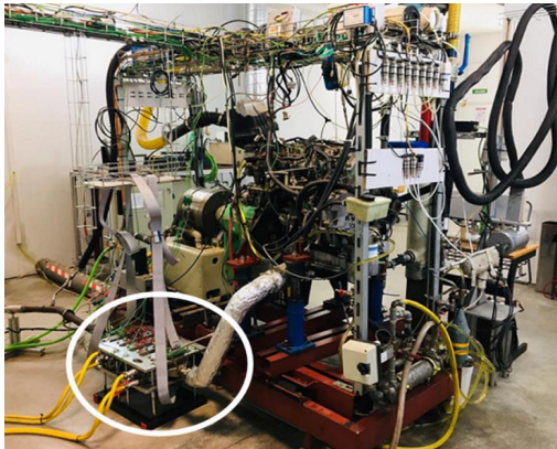
Figure 1: Experimental setup with TEG circled in white [1].
